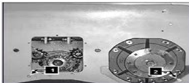
Fig. 3-8 Location of chaincase check plug (1) and rear drain plug (2).
