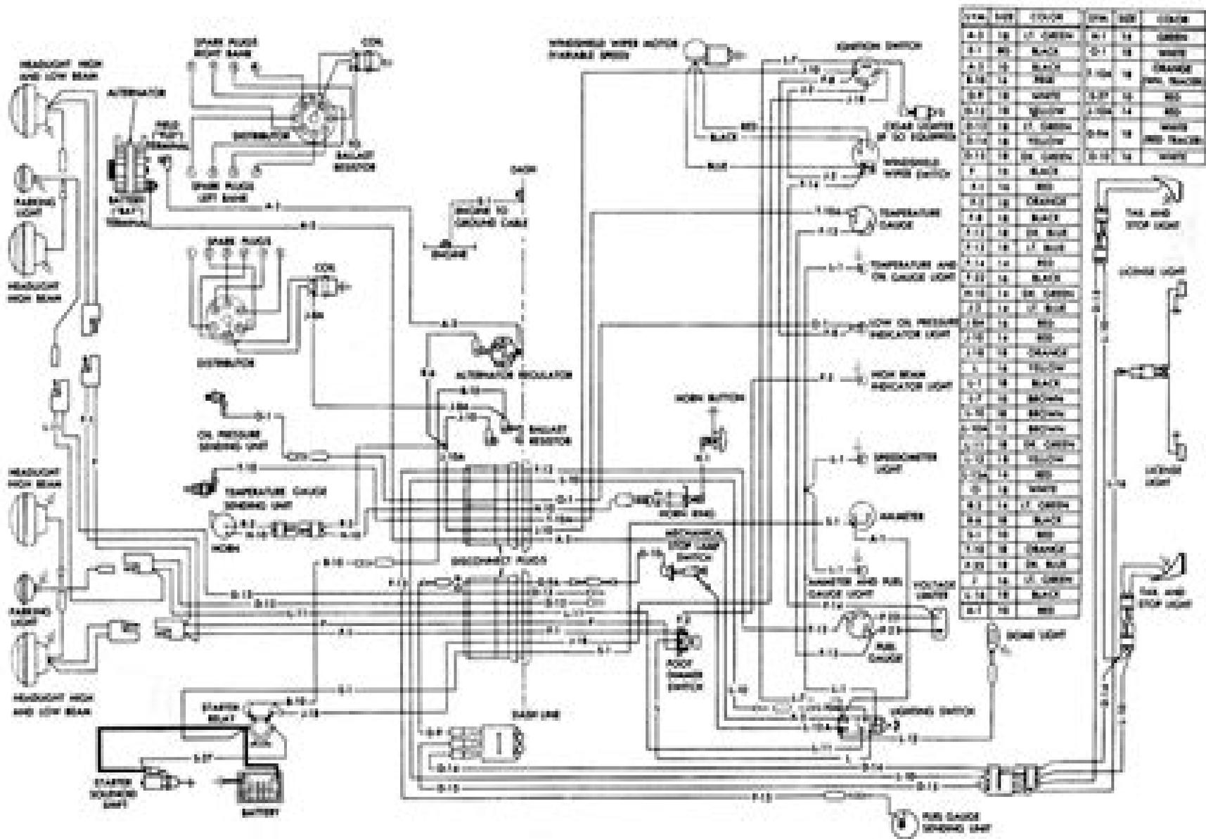
Fig. 9—Wiring Diagram—Town Panel and Town Wagen—D100, W100
