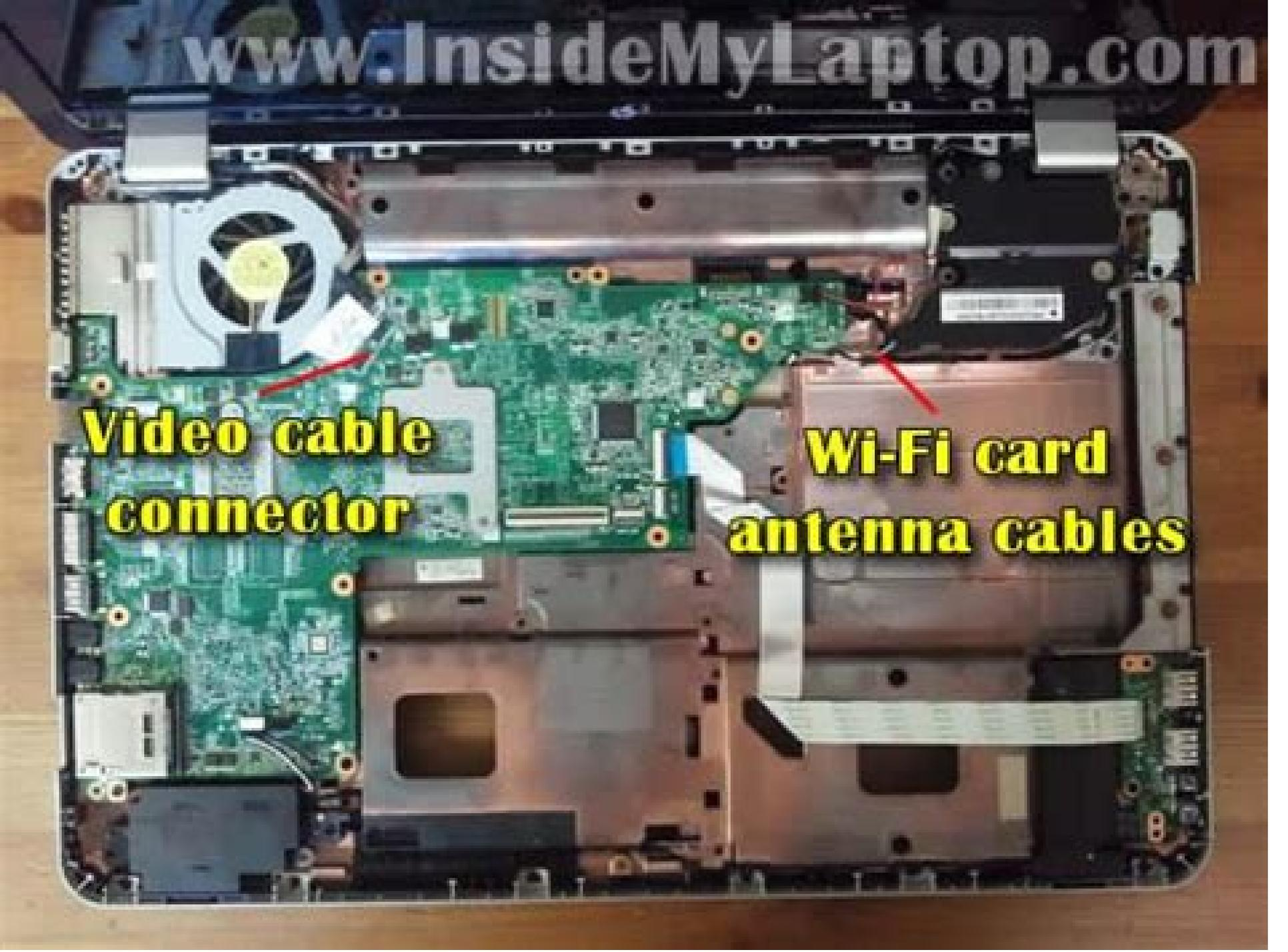
The image shows the internal components of a laptop with the bottom cover removed. A green motherboard is visible, with various components connected to it. A cooling fan is on the left, and a hard drive is on the right. Two red arrows point to specific connectors on the motherboard. The text 'Video cable connector' is overlaid in yellow on the left, and 'Wi-Fi card antenna cables' is overlaid in yellow on the right. The laptop is placed on a wooden surface.
