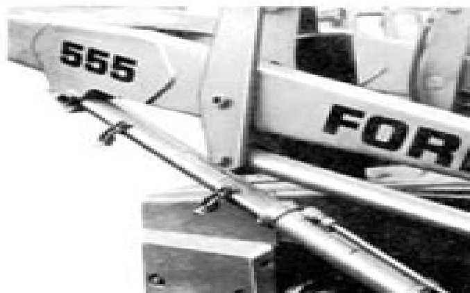
Figure 1 Loader Lift Cylinder "Safety Bar" Installed in Raised Position
