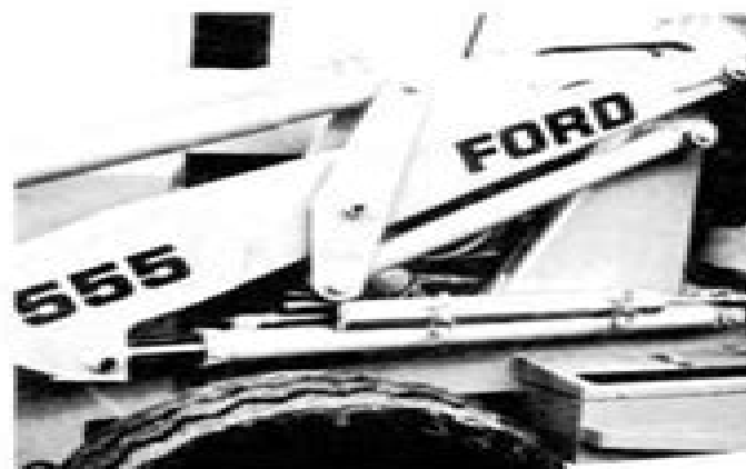
Figure 2 Loader Lift Cylinder "Safety Bar" Installed in Storage Position
