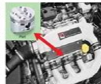
Figure 1-4 An assembly is a group of parts that work together to perform a function. For example, an engine is an assembly that contains pistons, which convert the fuel’s heat energy into usable kinetic energy (motion). As you will learn, an engine has many other parts. (Datum)
