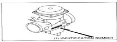
The carburetor identification number is stamped on the carburetor body.
