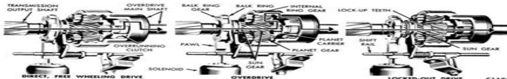
FIG. 6—Overdrive Power Flow
