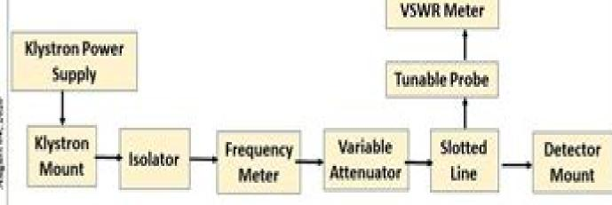
Block diagram of microwave test bench
