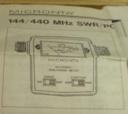
Your Micronta SWR/Power Meter is specifically designed for use with transceivers and antenna systems that operate on the 2-meter (144MHz) and 70-cm (440MHz) amateur radio
