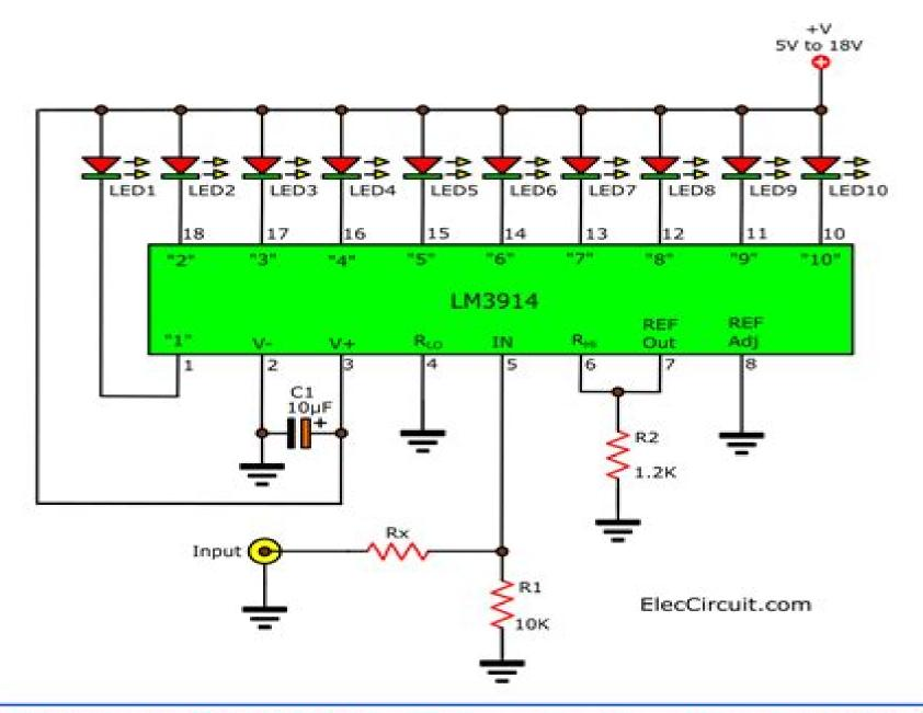
1.2V to 1000V Voltmeter circuit using LM3914
