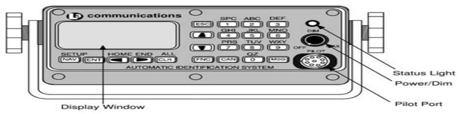
Figure 2-1. AIS Transponder
