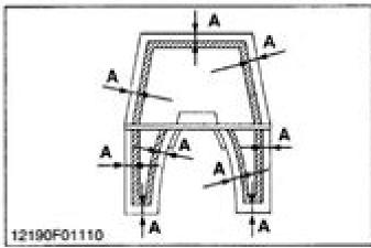
the waste which makes ethyl acetats and etc. to penet of cleaning area of the rear surface is indicated "A" if figure.
