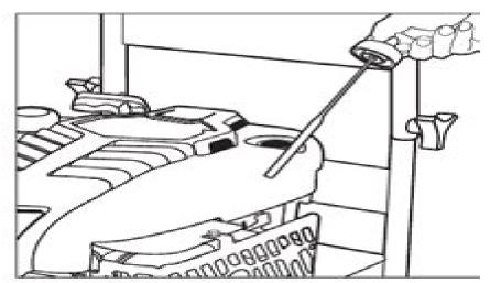
Step 2 Check oil level. Oil level should always be between the "FULL" and "ADD" marks on the dipstick. Be sure the machine is level when checking the oil level. (Refer to the engine's operating manual for seasonal grades.)
