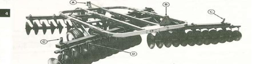
A-Leveling Crank B-Slow Moving Vehicle (SMV) Emblem (Attachment) C-Reflectors D-Combination Scraper
