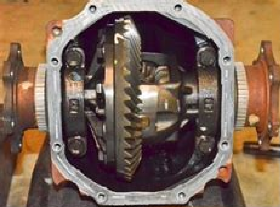
'07 350Z Base 6 Speed with the Open Diff, and 3.538:1 Gear Ratio
