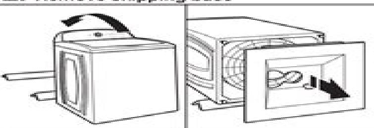
To avoid damaging floor, place cardboard supports from shipping carton on floor behind washer. Tip washer back and place on cardboard supports. Remove shipping base. Set washer upright.
