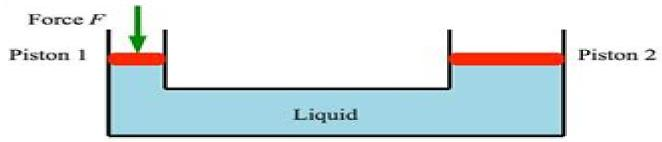
A hydraulic press is built as shown in the side view above, with a closed container filled with a non-compressible liquid. A circular movable piston on either side of the container allows force to be exerted on the liquid. In the diagram above Piston 1 has a diameter d and Piston 2 has a diameter 2d. When a downward force F is applied to Piston 1
