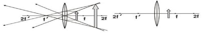
6. Camera lenses are described in terms of their focal lengths. A typical 35 mm (the size of the film) camera has a 50.0 mm lens. This means that the focal length of the lens is 50.0 mm. If the camera is focused on an object that is 3.00 m away, what is the image distance?
