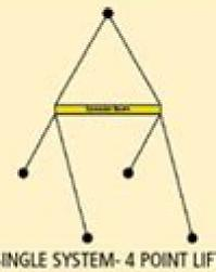
SINGLE SYSTEM- 4 POINT LIFT A single beam with the load being lifted at four individual points.
