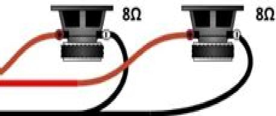
Speakers connected in parallel divide their impedance (Total Ohms):  $8\Omega / 2 = 4\Omega$
