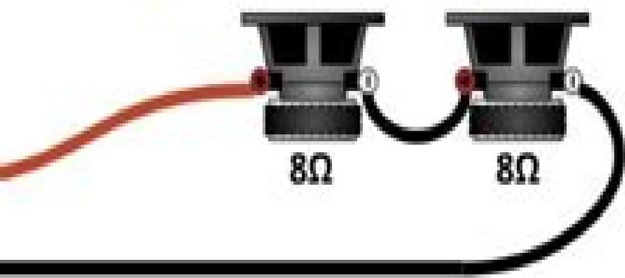
Speakers connected in series add their impedance (Total Ohms):  $8\Omega + 8\Omega = 16\Omega$
