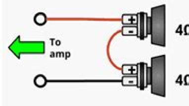
Series speakers: The speaker ohm values are added together. Each speaker gets only ½ of the amp power output.
