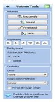
You can use Volume tools to quantify the signal intensity of bands, spots, arrays, and other image data. Define an area of interest by surrounding it with a shape. You can choose a rectangle, circle, freehand, or lane shape by clicking the appropriate button under the Volumes field.
