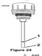
Note: The oil level on the dipstick will be incorrect if the oil is checked when the unit is hot.
