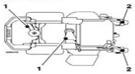
Lubricate front caster pivots once a year. Remove hex plug and cap. Thread grease zerk in hole and pump with grease until it oozes out around top bearing. Remove grease zerk and thread plug back in. Place cap back on.
