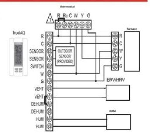
IF A THERMOSTAT OTHER THAN A TH5110, TH5220, TH5320, TH6110, TH6220, TH6320, TH6110, TH6320 OR TH6321 IS USED, A RELAY MAY BE REQUIRED TO
