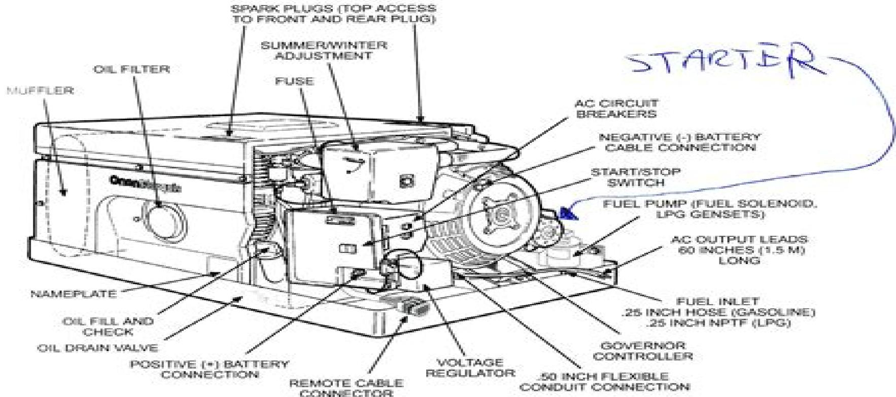
**FIGURE 7-5. BGM/NHM GENERATOR SET (ELECTRONIC-GOVERNOR VERSION)
