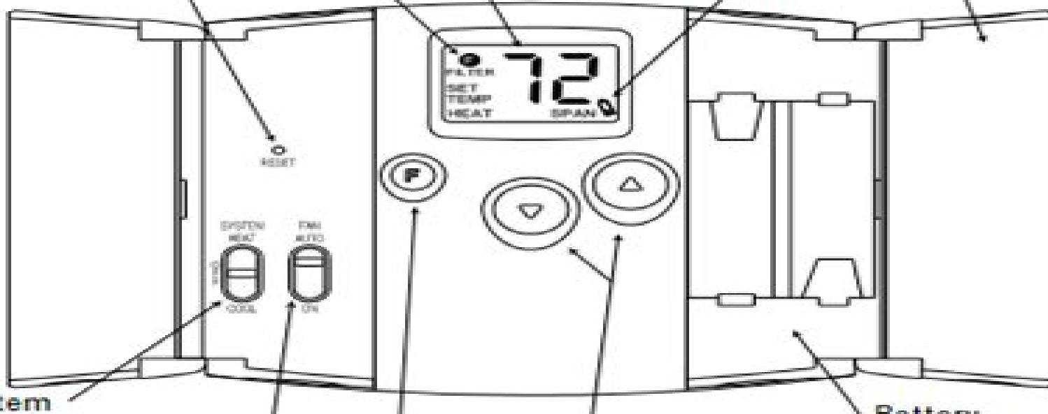
**System Switch:** Selector switch for Heat, Cool, and Off.
