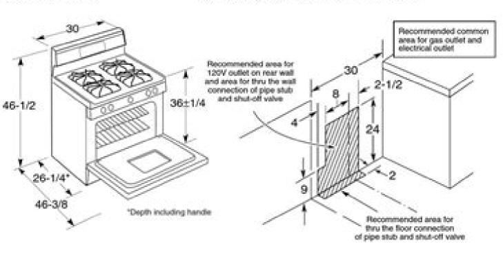
Installation Information: Before installing, consult installation instructions packed with product for current dimensional data.
