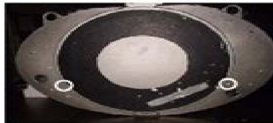
FIGURE 3 - SCREWS SECURING JOYSTICK ASSEMBLY TO BASE
