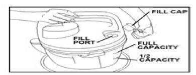
Remove fill cap. For a **full tank** of cleaning solution, pour 2 oz. of detergent into tank through fill port and fill tank to "full capacity" ine (1/2 gallon) with hot tap water.
