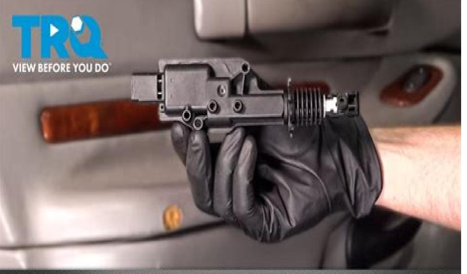
HOW TO REPLACE REAR DRIVERS SIDE DOOR LOCK ACTUATOR
