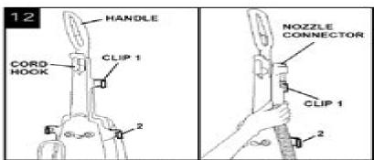
To store hose on rack, begin by placing nozzle connector end of hose (straight end) into clip 1 on rack (Fig. 12).
