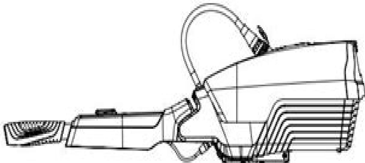
• Step 1: Pull the trim release lever and tilt up the outboard.
