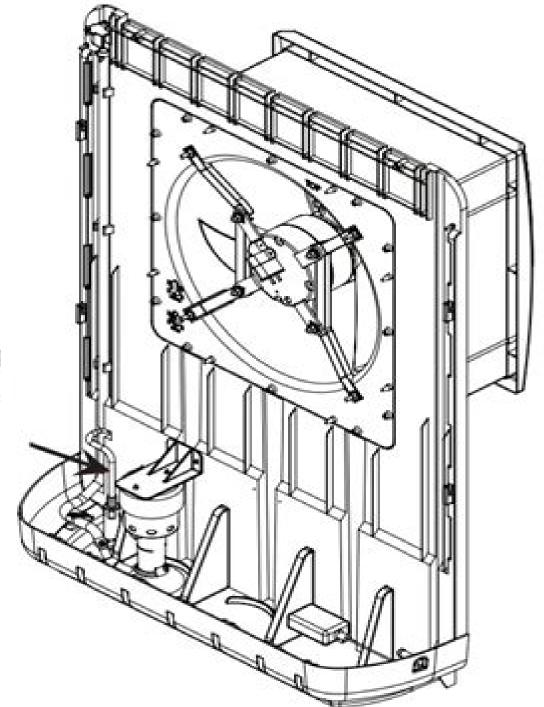
Remove and discard existing water hose. Replace with long hose from kit.
