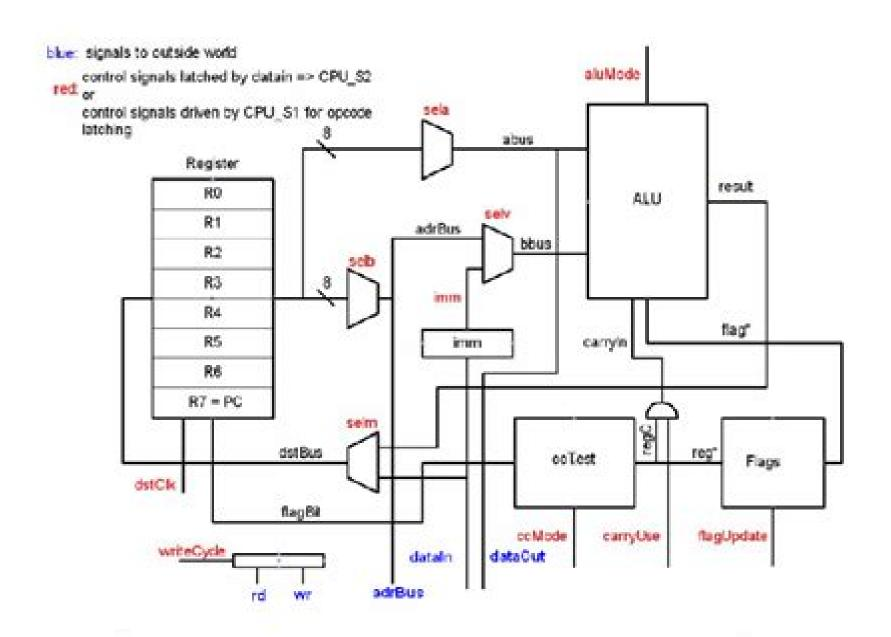
Figure 3. Data path for 64-bit RISC Processor [5]
