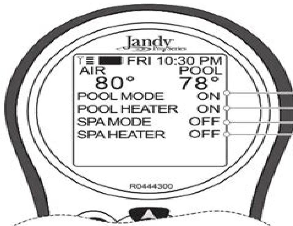
If the wireless handheld remote is part of an AquaLink PDA system, additional setup and programming options are available from the remote user interface (UI).
