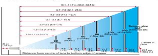
\* When installing against a wall, leave a space of about 20cm (7.9 in.) between the projector and the wall.
