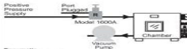
Figure 2. Chamber Evacuation below Atmosphere
