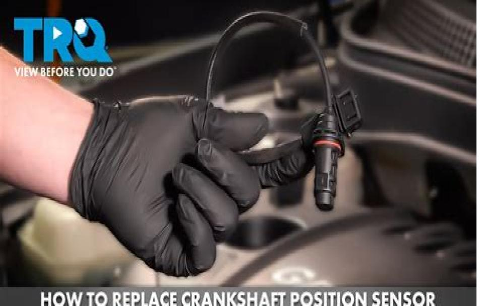
HOW TO REPLACE CRANKSHAFT POSITION SENSOR 2011-2014 HYUNDAI SONATA (2.4L L4)
