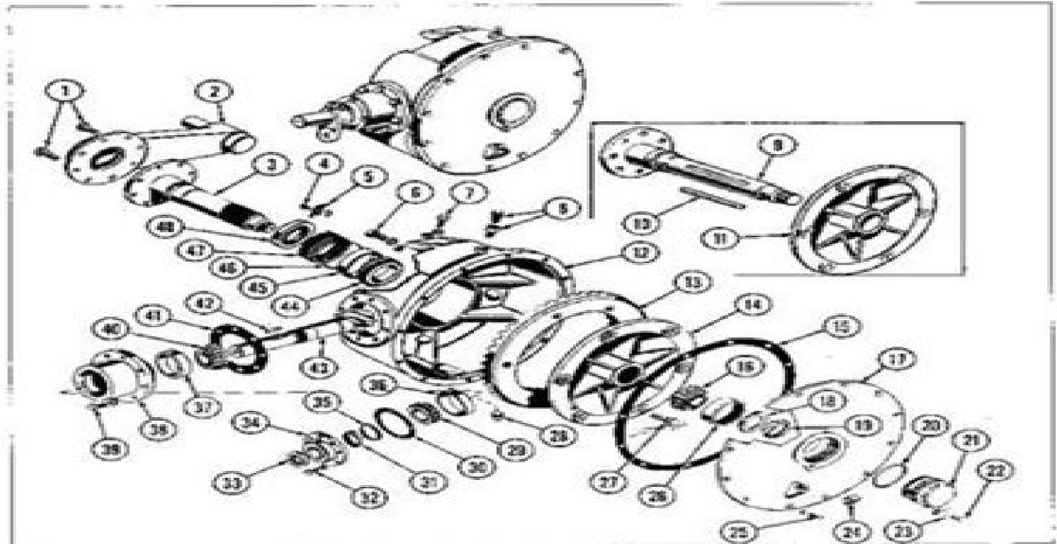
Fig. 1 — Bevel Gear Main Drive Assembly
