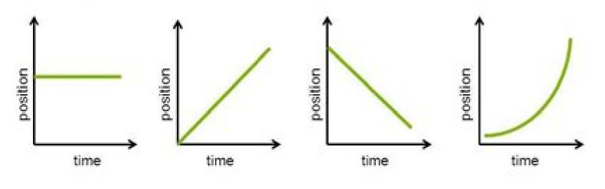
Slope is zero ∴velocity is zero (object at rest) Slope is positive :velocity is constant, positive Slope is negative .:velocity is constant, negative Slope is curve .:velocity is **not** constant (object accelerating)
