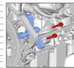
To prevent conducted extense, install EN-69792 lacking tool (2) and starter motor belon (1) at the starter motor income and engaging the Emplote.
