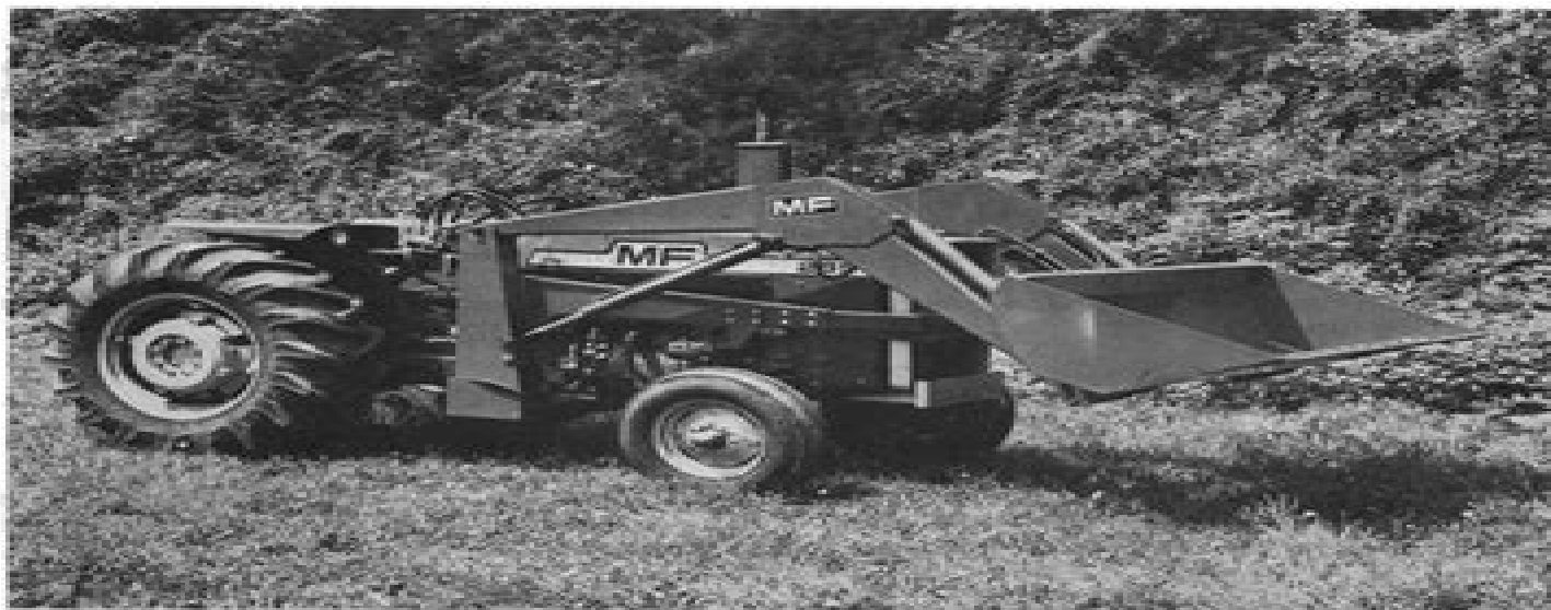
MF 265 Tractor and Loader Mounted Control Valve and PTO Pump
