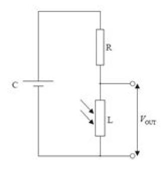
A photoresistor or light-dependent resistor (LDR) or photocell is a light-controlled variable resistor. The resistance of a photoresistor decreases with increasing incident light intensity; in other words, it exhibits photoconductivity. A photoresistor can be applied in light-sensitive detector circuits, and light- and dark-activated switching circuits.
