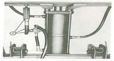
Remove plug from end of hydraulic cross and plastic plug from marker control valve. Attach 17-1/4inch (440 mm) hydraulic hose to marker control valve and hydraulic cross.
