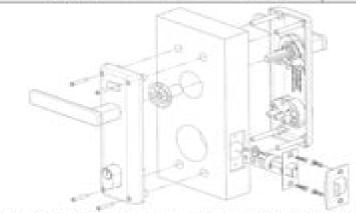
NOTE: The connecting Serve has 2 Armer, when installing aroune one Armer is pointing servicely North to 12 o'clock position and the other Arrow's printing horizontally towards the Soor Edge where the Latch's installed. His will arrow around and positive Privacy Button tocking function when dispressed.
