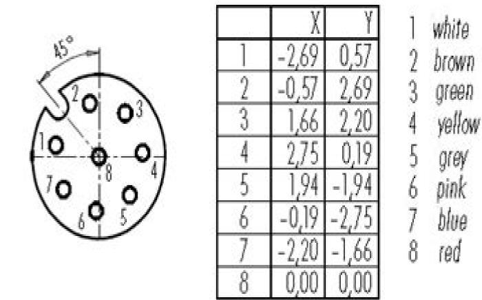
Shielded versions: shield on housing or pin 8
