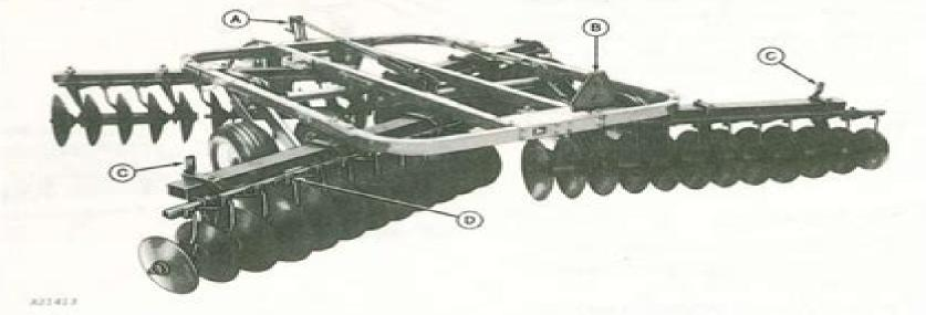
A-Leveling Crank B-Slow Moving Vehicle (SMV) Emblem (Attachment) C—Reflectors D—Combination Scraper
