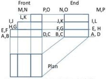
Fig 14 a First Angle projection of Fig 13
