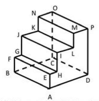
Fig 13b Isometric View (Hidden details)
