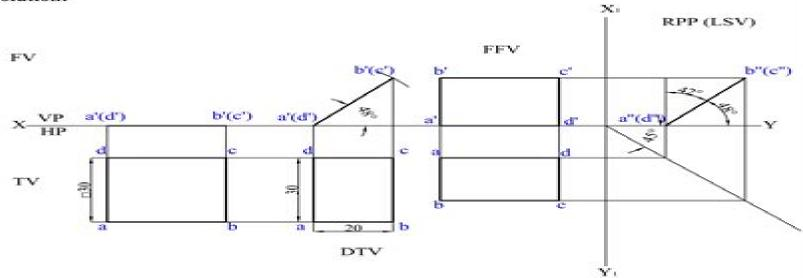
**Problem 17:** A rectangular lamina of 30mm x 20mm rests on HP on one of its shorter edges. The lamina is rotated about the edge on which it rests till it appears as a square in the top view. The edge on which the lamina rests being parallel to both HP and VP. Draw its projections and find its inclinations to HP and VP.
